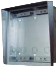
9135362E Roof & box for masonry fitting - 2 modules 229 x 240 x 41 mm Hole: 210 x 220 x 50 mm
