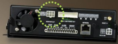
Additional power supply for cameras and Monitor
