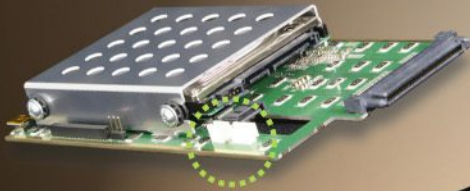
Attached M/B with built on heating architecture for both system and HDD
