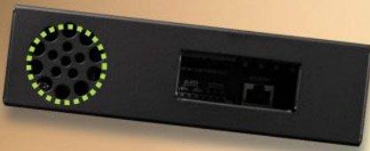
Additional Ventilation holes for heat management
